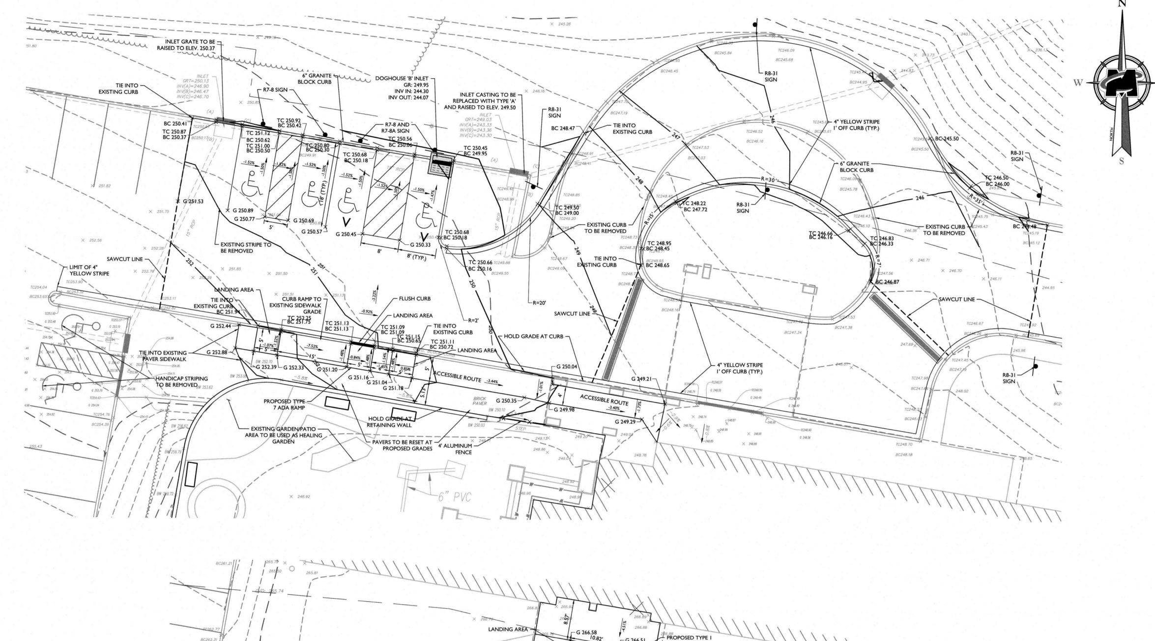
**LEGEND** € TRAVERSE LINE, CENTER LINE 13+00 OR BASELINE (LABEL AS SUCH) 12+00 RIGHT OF WAY LINE **EDGE OF PAVEMENT** FACE BACK DEPRESSED CURB A . A ... SIDEWALK ——X———X—— **FENCES** —x——x mmmm mmm MUNICIPAL BOUNDARY LINE STALL COUNT ADA ACCESSIBLE STALL DEPRESSED CURB AND ADA RAMP DIRECTION OF TRAFFIC FLOW SAWCUT LINE **BITUMINOUS** CONCRETE PAVEMENT FIRE FYDRANT RETAINING WALL LIGHT POLES
